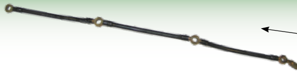
7570 Leak Off Pipe Fiat
