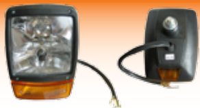
Head Lamp JCB New Type c/o bulbs and 30cm Fitted Cable
