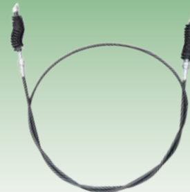
Throttle Cable JCB Telehandler 526-55 5205 5265 533-105 520-55 540 OE Ref: 331/14325
