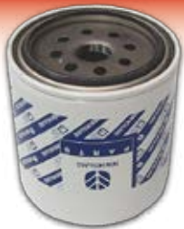
3751G ** USE 3751R WHEN STOCK IS GONE ** Engine Oil Filter Ford TW Genuine **8530 - 8830**7810 - 8210**
