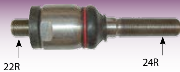
3144 Ford 40 'S Carraro 4WD Ball Joint (Right Hand Thread)
