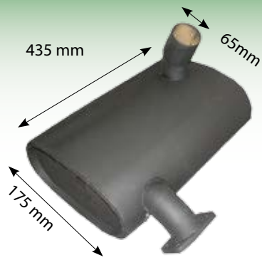
42004 Exhaust Box Ford TS115 Non Turbo For Corner Post Only
