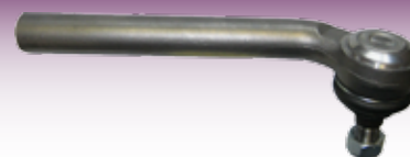
Ball Joint = 2825 404285 82/8340 R.H.Tre Track Rod End Ford 8200 8340 RH Carraro Axle
