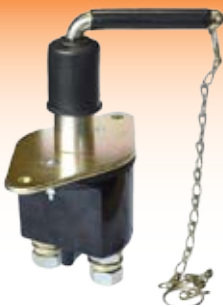
3875E Cut Off Isolation Switch Amp Heavy Duty Max Peak Load 12/24V 2500A for 5 Seconds Max Continuous Load 12/24V 250A OE Ref: 1939387
