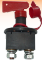
3875E Cut Off Isolation Switch Amp Heavy Duty Max Peak Load 12/24V 2500A for 5 Seconds Max Continuous Load 12/24V 250A OE Ref: 1939387
