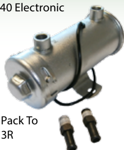
41613R Fuel Lift Pump Ford 60 M TM110-140 Electronic
