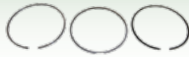
Q8094845 Ring Set Turbo Standard NEF Iveco Engine Case New Holland T4000 T5000 T6000 T9000 OE Ref: 8094845
