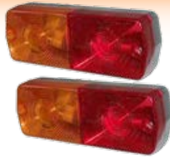
1716 Rear Combination Lamp 12v Flat PAIR 185mm x 67mm x 50mm
