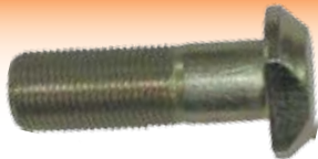
409750 Wheel Nut Ford 40 M TS Rear 3/4" UNF 8 per Hub
