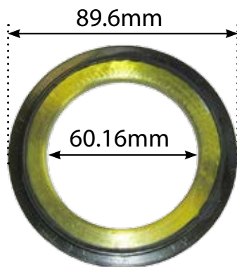
59304 Oil Seal Front wheel hub John Deere 20 30 40
