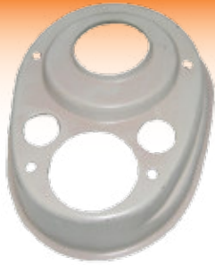
41796 Dash Panel Dexta **Holes for gauges**
