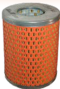
Fuel Filter 20D 35 65 Length 82.5 OD 71.00 ID 33.5
