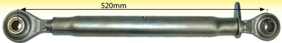
1689 Top Link 20" Cat 2 Tube 20" Adj. Min 25 3/32" Max 36 7/32"
