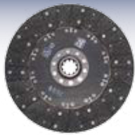
4106 Clutch Disc Fordson Super Major 12" Main
