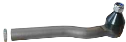
53733 Track Rod End Deutz Agrotron 100 110 80 90 - Left Hand 343mm long 24 x 1.5 RH Thread 25/27mm Taper 4.70 4.80 4.85 4.90 4.95 6.01 K90 100MKIII 105MKIII 80MKIII 85MKIII 90MKIII OE Ref: 04415653
